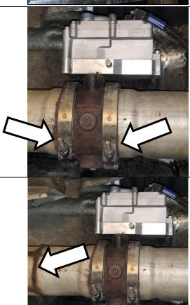
Weld the front adapter to the exhaust pipe. This weld must completely seal the exhaust system as it must retain pressure.
