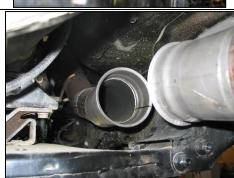
Install the brake valve between the two exhaust pipe adapters using the two supplied V-band clamps. Ensure the exhaust pipe adapters are in line with the brake valve to prevent possible leakage.
