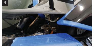
WITH THE HOOD OPEN, USE MASKING TAPE TO PROTECT EDGES OF HOOD AND FENDER THAT MIGHT GET SCRATCHED OR CHIPPED WHILE DOING THE FOLLOWING WORK.
