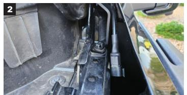
LOCATE AND REMOVE THE BODY END, REAR MOST HINGE BOLT. BOLT IS REUSED FOR BOLTING DOWN THE BRACKET.
