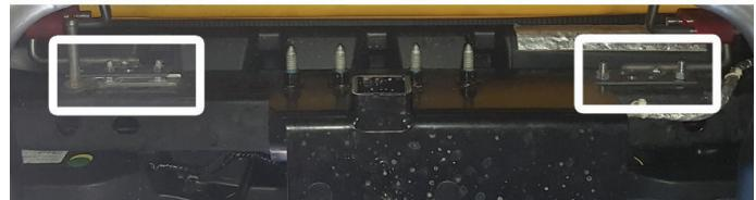
6. Connect **muffler (1)** to mid pipe, inserting wire hanger into rubber hanger. Adjust muffler to fit properly as shown then tighten clamp.
