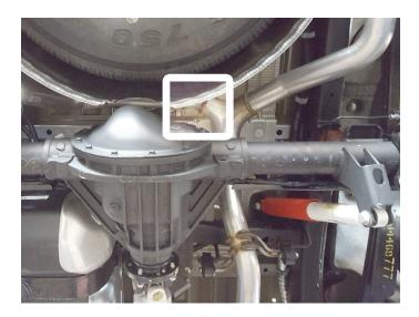
4. Remove bolt and mount securing driver side tailpipe then remove it from vehicle. Retain bolt and mount for later use.
