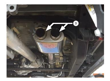
13. Route **right front tailpipe (5)** and **left front tailpipe (4)** over axle and connect them to muffler outlets. Mount wire hangers into isolators then tighten clamps (x2) enough to allow for adjustment.
