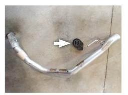
5. Cut tailpipes just behind factory muffler.
