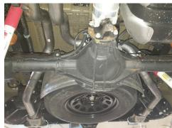
16. Adjust exhaust components for fit; maintaining ½" clearance and compensating for suspension, travel and vibration then tighten all clamps. Finally, fit (x3) hanger keepers (10) onto each sideways hanger.
