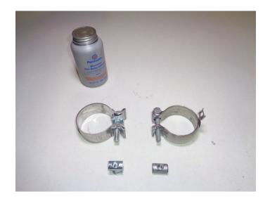
Place clamp (removed step 8) onto inlet pipe (1) then connect it to catalytic converter. Mount wire hanger into factory isolator and tighten clamp just enough to allow for adjustment.
