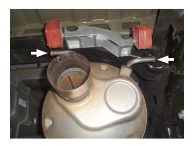
6. Remove nuts from factory pipe and catalytic converter flange. Remove muffler and factory pipe from vehicle.
