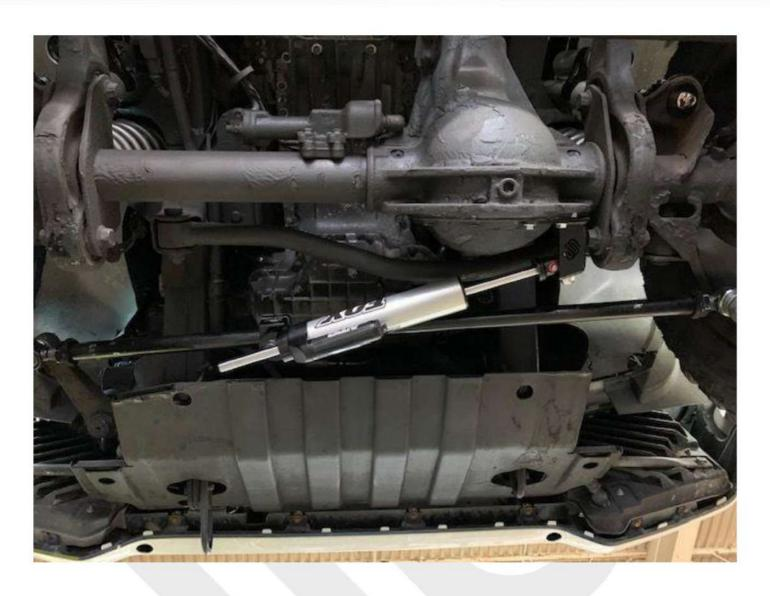
5. Install the large bolt on the differential side next. You can torque this bolt completey at this time.
