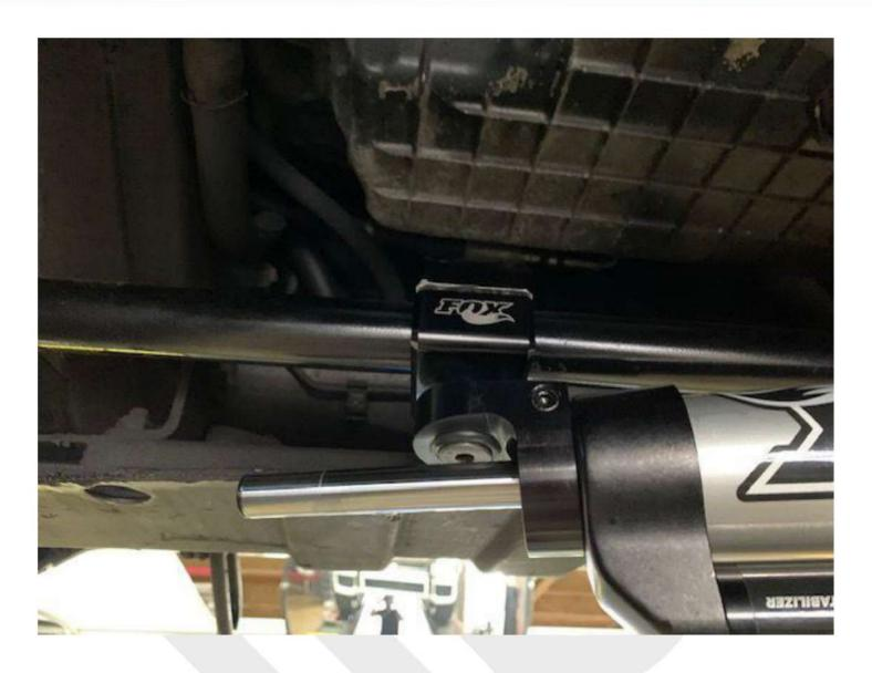
4. If you measure from the end of the locking nut at the pitman arm. You will be approx 12.5 inches from end to end. this will cause no binding issues turning lock to lock from left to right.
