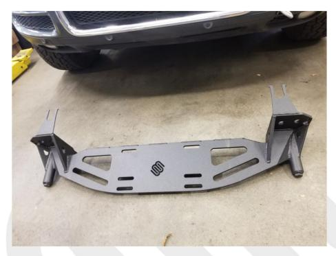
Remove 4 mounting bolts on each side (8 total) for the OEM bumper reinforcement.
