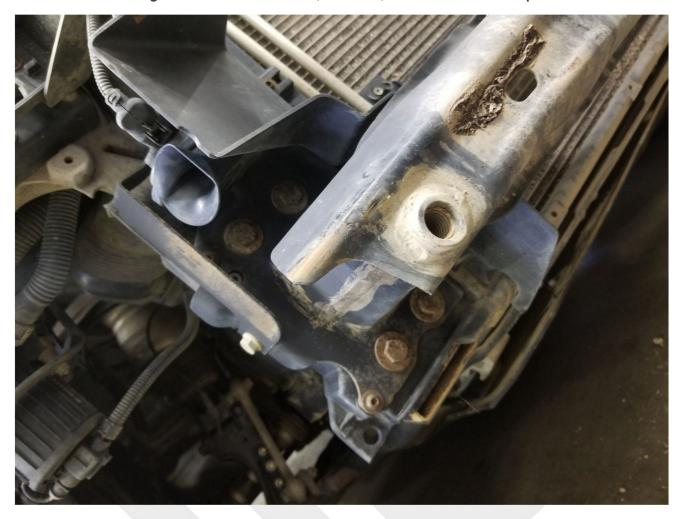
Remove OEM horn mounting bracket and it will be transferred onto the new hitch mount.
