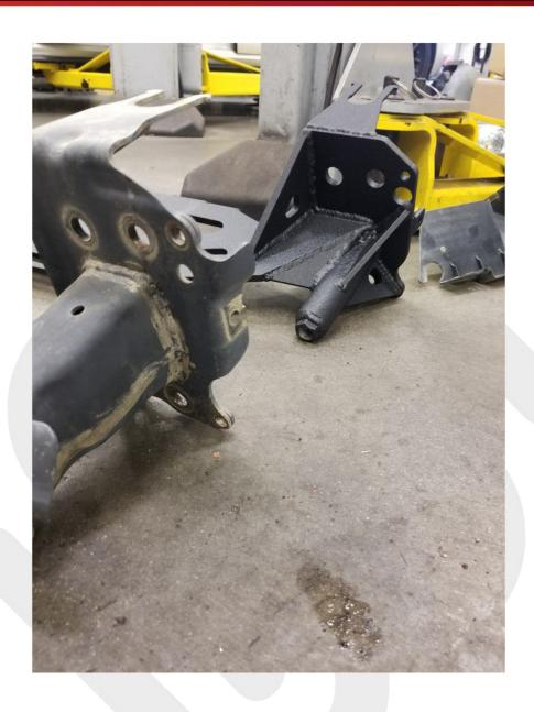
There is a clip on the radiator mount that is built into the OEM hitch mount. This needs to be unclipped from each side to remove the OEM bumper support. The new one will be installed the same way as the OEM. Using some lubricant on the radiator mount bushing will make reinstallation easier.
