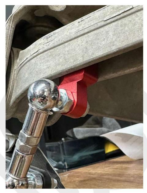
Install supplied level sensor relocation link as shown above. It replaces the front upper control arm level sensor bracket. It will reposition the arm back so there is no binding with the new shorter arm. It will also reinforce the OEM plastic arm as they are prone to breaking due to being plastic.
