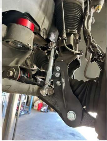
On the subframe there are two aluminum tabs that will contact the lower airstrut magnetic sensor. These tabs need to be broken or cut off, they are aluminum so a saw will cut thru them easily. Or you can use a cut off wheel and cut the surface and then use a hammer to knock it off the rest of the way.
