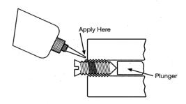
Avoid touching the bottle tip to the metal surface. Not recommended for pre-assembled threads in a blind hole.
