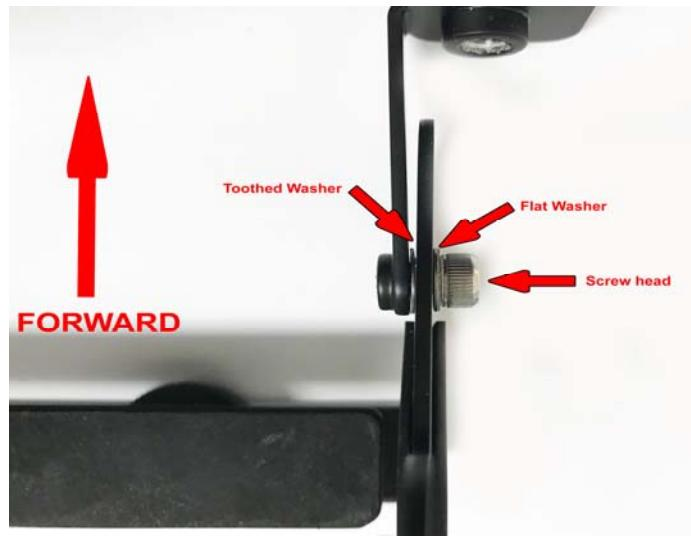
**Step 2D** - With the plate holder on hand tight, determine your final position and tighten the mounting screws using the Allen head (hex) tool provided.
