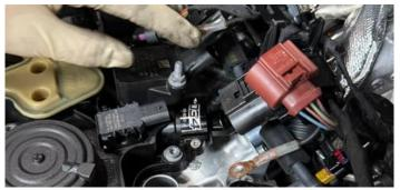
**Step 10:** Grab the second -10 AN hose and route as shown. The 90 deg connection is used to attach onto the fitting you just installed. Be careful when routing the hose and not to damage any sensor cables. Tighten the connection with a -10 AN wrench. This AN hose goes to the "IN" port of the catch can.
