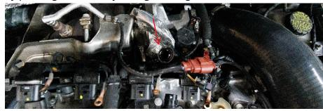
**Step 8:** At this point, you can insert the -10 AN hose with the new Norma connetion onto the PCV hose you just relocated. (This hose goes to the "OUT" port of the catch can.
