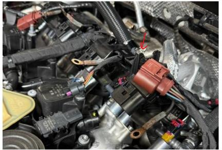
**Step 9:** We now have a 45 degree billet fitting to insert into where we removed the PCV hose from. It is secured into place by the two billet halves and the M4 bolts. Use a 2.5mm Allen bit or Hex to tighten the halves, rotating the assembly as needed to tighen both ears. **Be very careful not to drop the M4 bolts into a crevice or the spark plug hole.**
