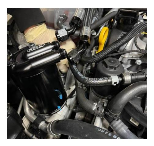
**Step 15:** Reinstall the catch can. Torque the mounting bolt to 40Nm + 90 degrees.
