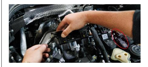
**Step 4:** Remove coil pack#4 (the coil closest to the intake) by completely removing the 10mm stud holding it down. A coil puller tool can help remove the ignition coil.
