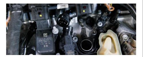
**Step 7:** Carefully route and position the PCV hose as shown below by pushing it under any wiring / hosing.
