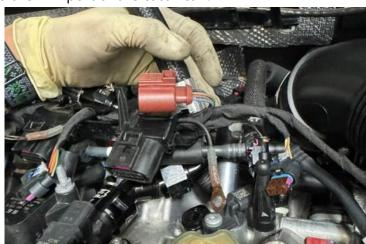
**Step 11:** At this point, we need to plug in everything we have removed in reverse order (the three camshaft solenoids, the pressure sensor, the ground straps on the ignition coil studs), **but first:**
