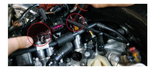
**Step 6:** Remove the PCV connection from the housing by gripping the tabs and pulling away. The flat head can help here to carefully pry the connection off of the housing.
