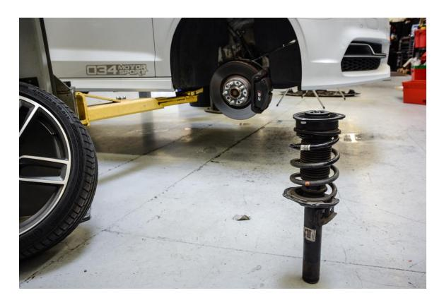
**Step 17 -** Reinstall the strut assembly and loosely thread the upper 3 strut bolts into strut mount.
