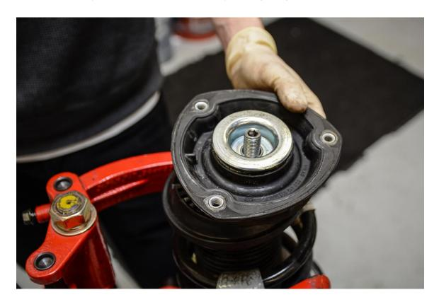
**Step 14 -** Install new 034Motorsport Street Density Strut Mount and, if desired, new Strut Bearings. Locate tab on strut mount and align with recess in upper spring perch.
