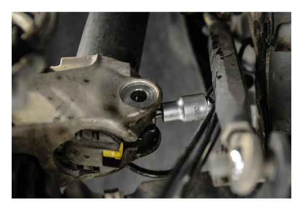
**Step 10C** – Once lower strut bolt and nut are removed, use a Spreader Socket to separate the strut housing from the lower knuckle. Spreader Socket shown inserted into lower knuckle below.
