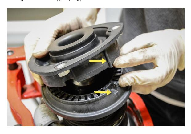
**Step 15 -** Once all mounting tabs are aligned, install upper strut nut **using a 21mm (or 13/16" Standard) Spark Plug Socket and 7mm Allen**. Torque upper strut nut to <u>60 Nm</u>. **Important:** For proper installation, the upper strut mount tabs must align with the tab on lower strut body.
