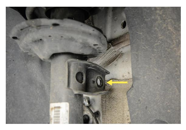
**Step 9** – Locate the bolt clamping bottom of the strut to the knuckle. Use a 14mm Triple Square and 18mm Socket to remove the nut and bolt from the knuckle assembly.
