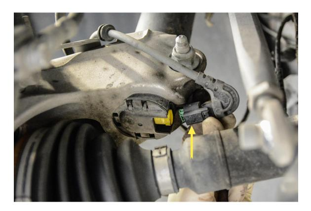
**Step 8** – Remove upper nut from front sway bar end link, located on bracket below spring perch of strut assembly. (If aftermarket sway bar end links have been installed, new hardware may have been supplied and will differ from factory pieces.) **Tip:** Remove upper sway bar end link nuts from both sides of the vehicle for added compliance when removing strut assembly.
