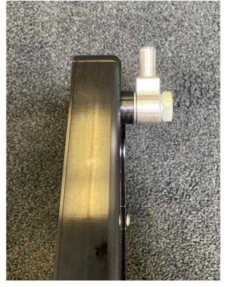
**Step 13** Tighten the banjo bolt to 20 NM, with the fitting outlet in this orientation.
