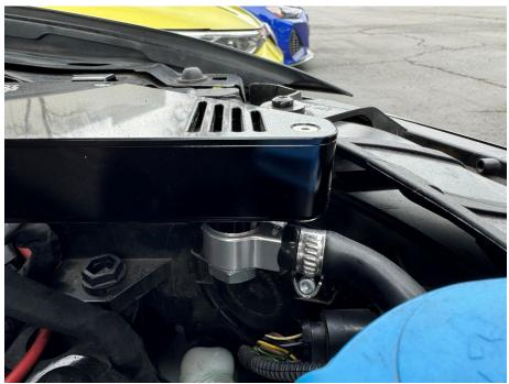
**Step 18** Reinstall your intake onto the grommets and secure the clamps with a 7mm socket/wrench.
