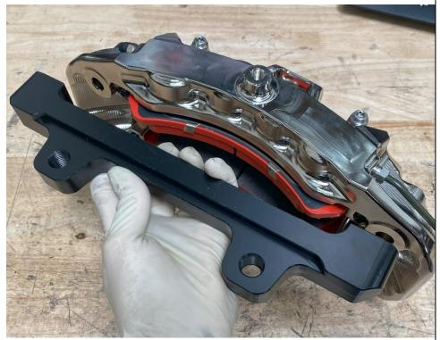
Using a 10mm Allen socket, torque the two supplied M12 bolts that attach this bracket to the caliper. The torque spec is 95Nm.
