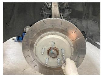
**Step 7:** Remove the rotor and set it aside. You should now have a bare wheel hub. Take a quick breather.
