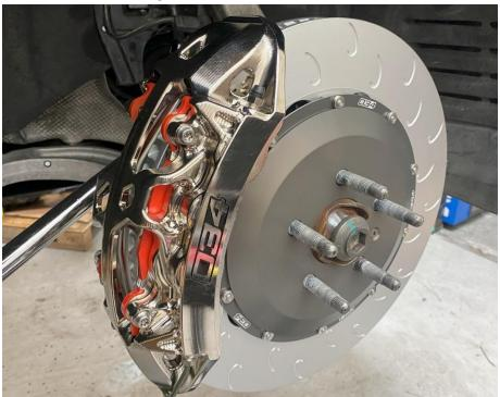
**Step 12:** Now that it's sitting on the rotor, align the bracket and wheel knuckle/hub holes. Using the supplied M14 bolts and a 12mm Allen socket, torque to 195Nm.
