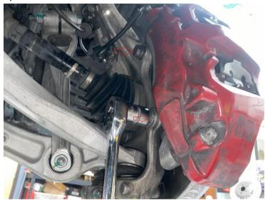
**Step 6:** Remove the caliper from the rotor and set it aside. Remove the rotor set screw with a T30 torx bit.
