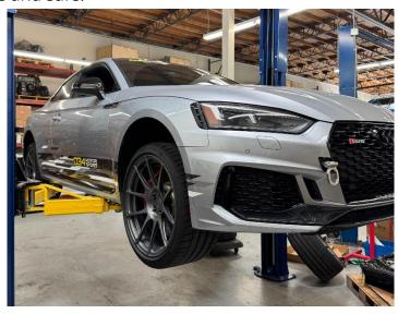
**Step 2:** Take the wheel off using a 19mm socket on the lug nuts (17mm for OE).
