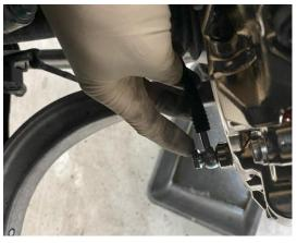
**Step 14:** Route the brake line as shown, making sure the grommets are clipped into their respective retainers.
