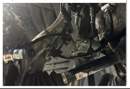
**Step 15:** Use an 11 mm wrench to button up the brake line to the OE hard line.
