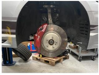
**Step 3:** Remove the brake line from the hard line with an 11 mm wrench. Make sure to cap it or have a bucket to catch the residual brake fluid.
