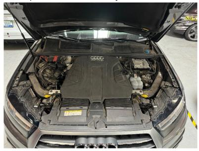
**Step 2**Remove the intake cover to reveal the intake filter.
