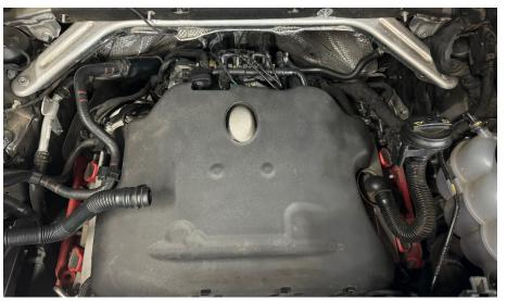
**Step 9**Remove the supercharger heat shield cover.
