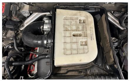
**Step 21**Reinstall the air box cover.
