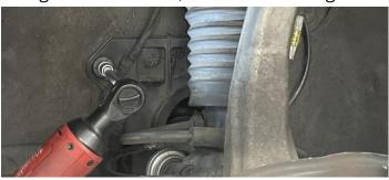
**Step 8**Unclip the ride height sensor harness.
