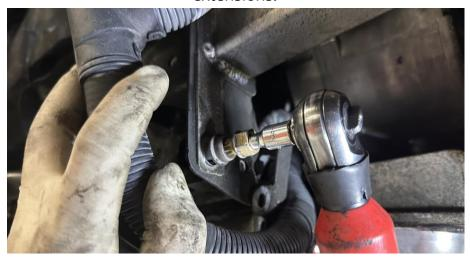
**Step 48**Reconnect the coolant pump.
