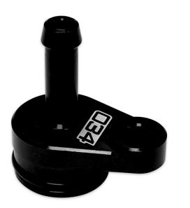
The 034Motorsport Billet Coolant Vent Union is designed to replace the factory plastic and failure-prone coolant union on the cylinder head of the EA888 Gen3 and Gen4 engines. Being next to the turbocharger, the factory plastic coolant union is subject to a lot of heat, becoming brittle and failing over time.
