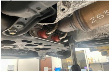
**Step 4**Using a 16mm socket, remove the dogbone mount hardware.
