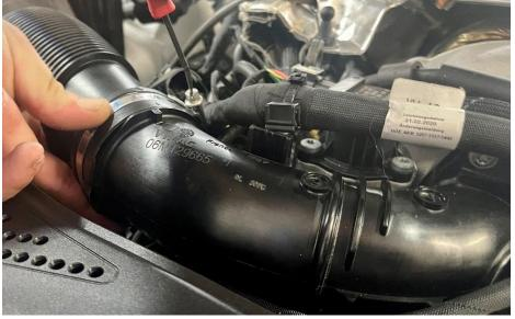
**Step 4** Slide the hose off of the turbo inlet.
