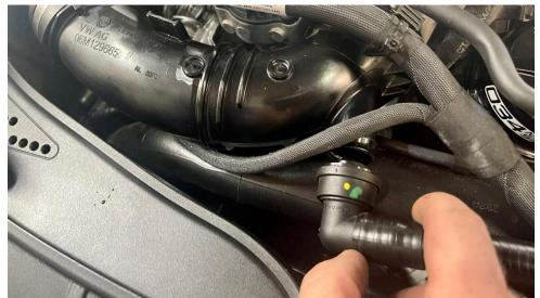
**Step 7** Using a T30 Torx, remove the factory hardware from the turbo inlet. The lower bolt is a bit tricky to reach.
