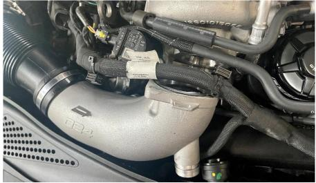
**Step 14** Using a 5mm Allen, tighten both bolts to secure the 034 turbo inlet to the turbo.
