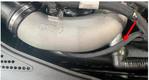
**Step 16** Attaching the vacuum line fitting to the turbo inlet is a bit tricky, take your time and push the fitting onto the turbo inlet. (Fitting is under the inlet)
