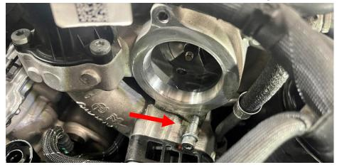
**Step 11** Apply a small dab of grease to the o-ring slot on the 034 turbo inlet. Install the o-ring into the slot. This will prevent the o-ring from falling into your engine bay.
