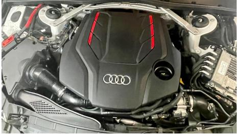
**Step 2** Remove the engine cover by pulling up on it.
