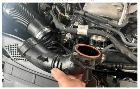
**Step 10** Install the lower bolt onto the turbo flange.
