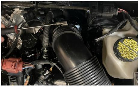
**Step 4**Remove the factory intake hose.
