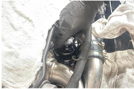
**Step 11** Using a 32mm socket, secure the housing.
