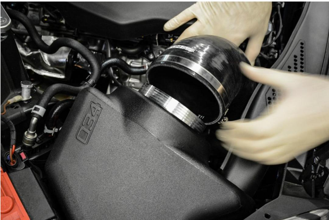
**Step 15** - Using an 8mm Hose Clamp Driver or Socket, tighten the lower hose clamp first, securing the inlet hose to the turbo inlet.
