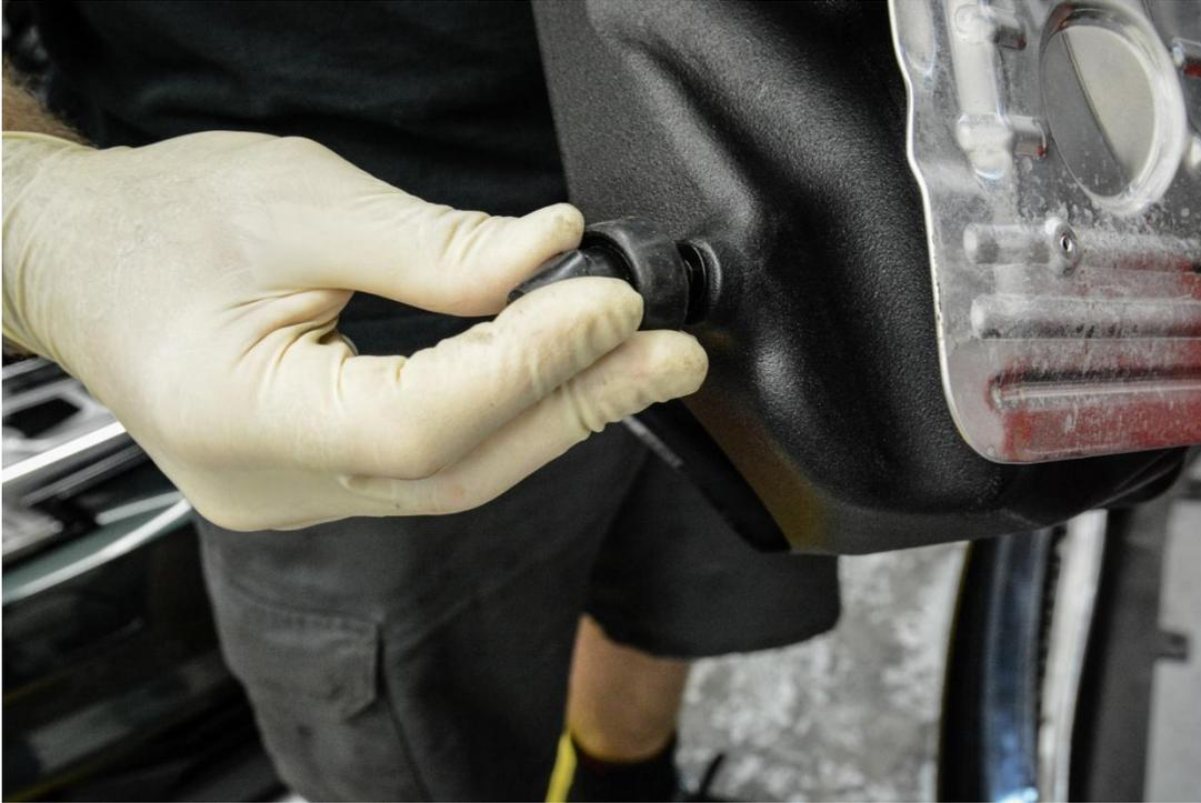
**Step 12** – Tip: Spray the rubber grommets with a lubricant to help them seat properly in the engine bay when installing the air box.
