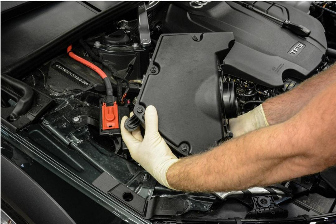
**Step 7** – The air box and intake tube should be completely removed now. Take a deep breath, and prepare to install your new P34 Cold Air Intake.
