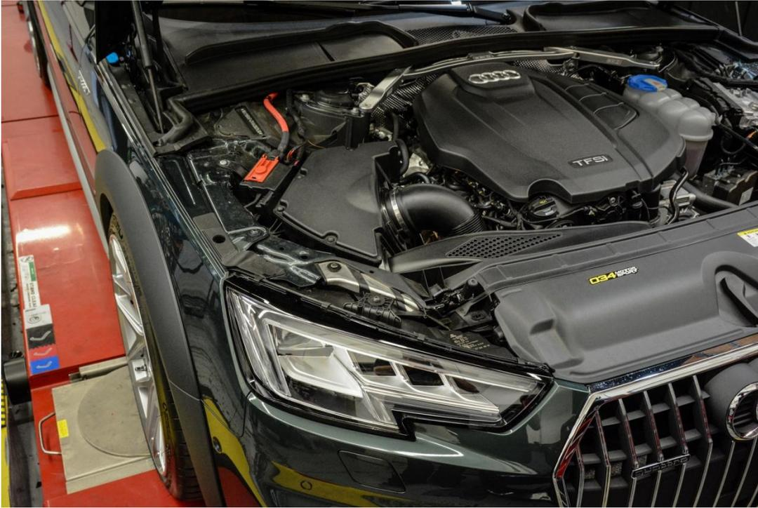
**Step 2** – Using a 7mm Hose Clamp Driver or Socket, loosen the hose clamp securing the intake tube to the turbo inlet.
