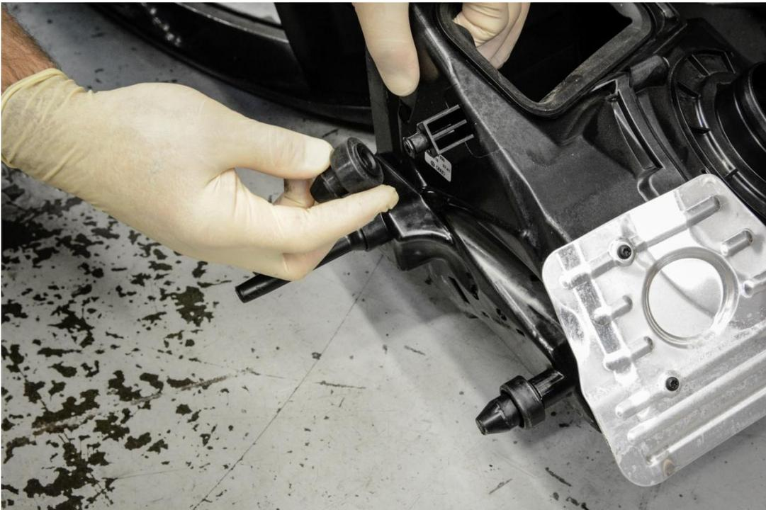
**Step 9** – With a T20 Torx, remove the 3 screws securing the heat shield to the factory air box.
