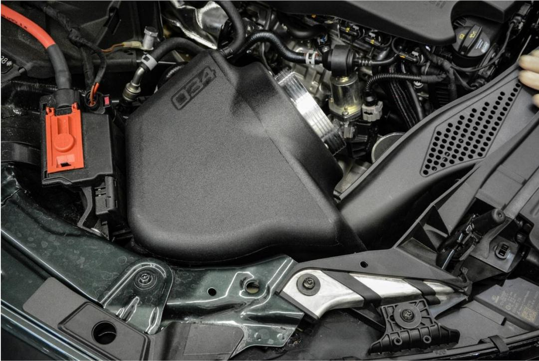
**Step 14** – Position the 034Motorsport Silicone Inlet Hose into place, seating the bottom of the hose on the turbo inlet and the upper portion on the air box. **Note:** Loosely pre-install the supplied hose clamps to the inlet hose before placing in the engine bay.
