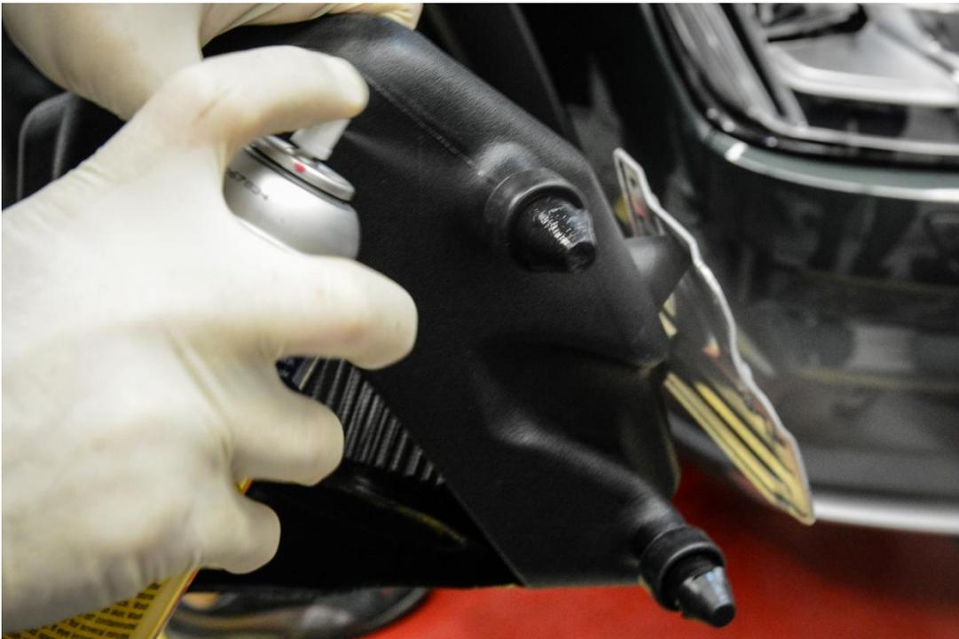
**Step 13** – Seat the P34 Cold Air Intake into place on the factory fresh air duct, then align with the holes for the factory mounting grommets. Push down firmly to fully seat the grommets.
