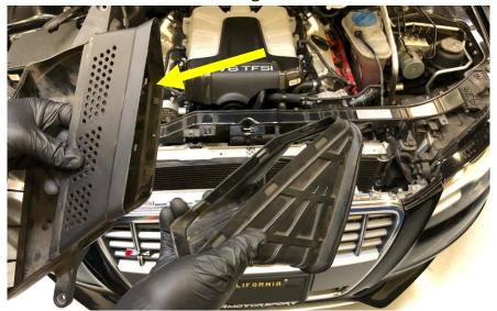
**Step 5**Remove the engine cover and set it aside.
