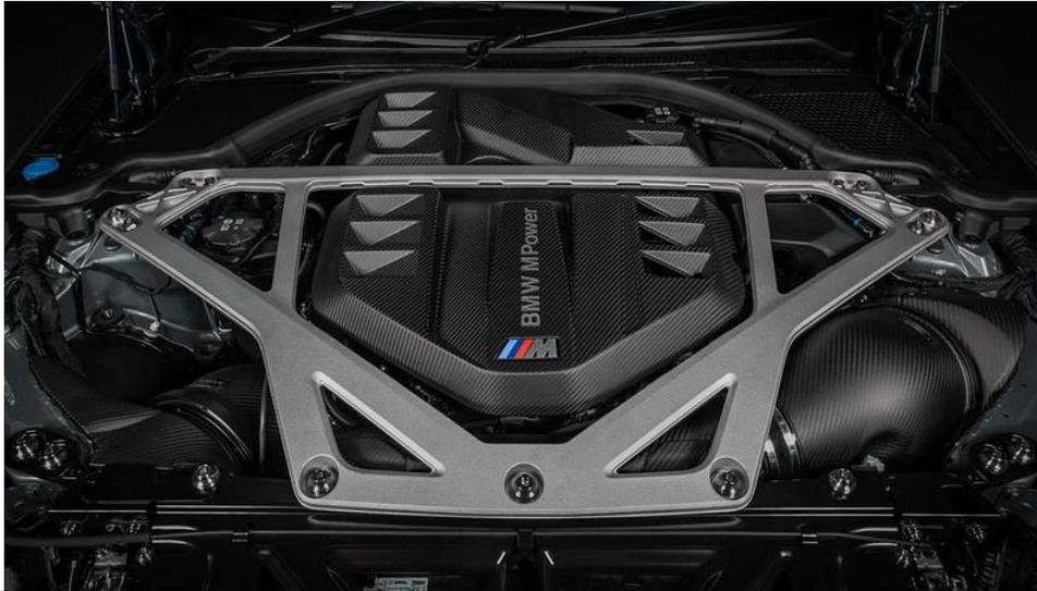
1. The vehicle **MUST BE** on the ground. Remove the stock brace using the 13mm and 17mm sockets. If you have an M2 please also remove edge seal and cosmetic covers
