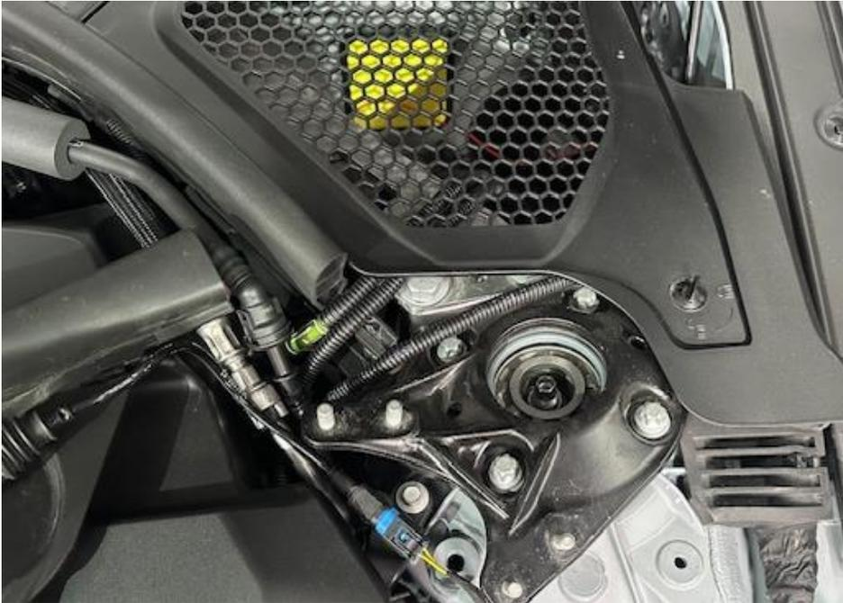
4. If the rear studs do not line up with the brace you will need to adjust the brackets around the strut supports on each side. Adjusting these will not affect vehicle alignment. Remove the trim covers over each strut.
