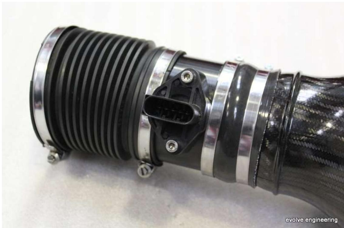
13. Fit Evolve Carbon housing into silicone hose and tighten the hose clamp shown in the picture shown. (Ensure orientation of the MAF sensors to the plaques is as shown for both banks):
