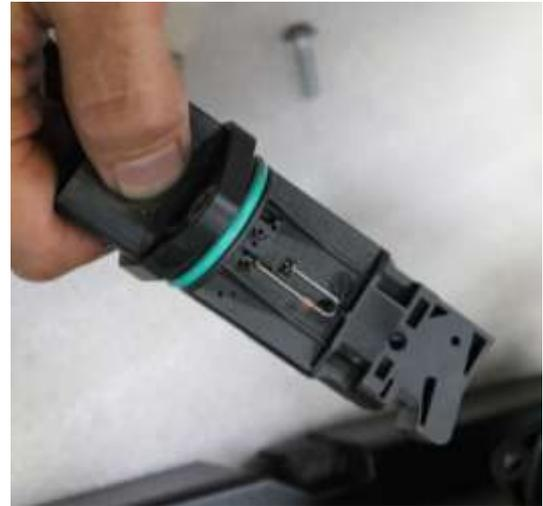
10. Insert MAF sensors into Evolve MAF housings using supplied bolts
