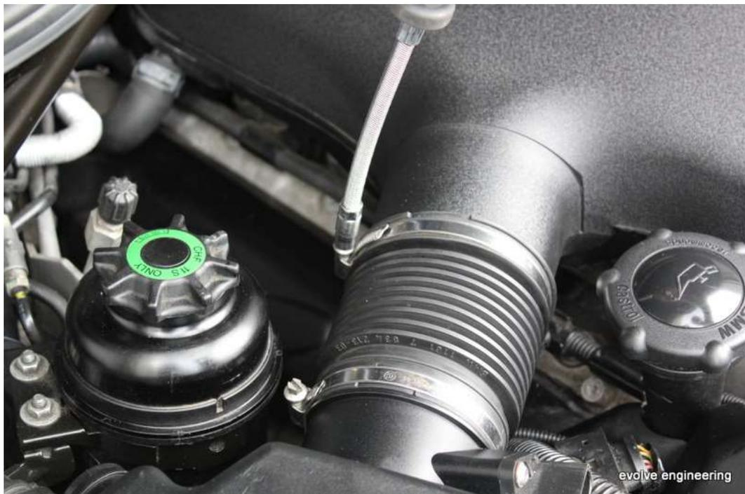
4. Remove lower air box assemblies. Bank 1 requires 10mm socket, bank 2 require T30 Torx
