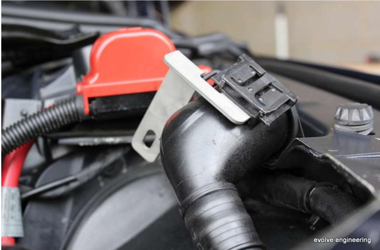
26. Secure bracket to right side panel using supplied flanged bolt and nut as shown:
