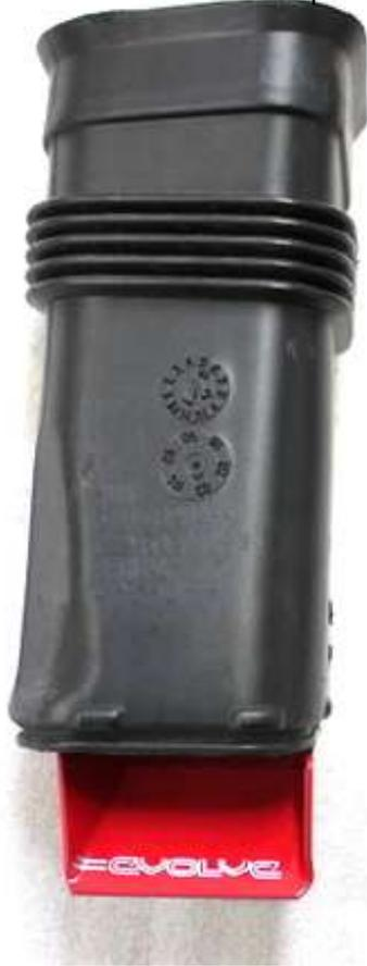
Ensure the scoop is forward facing once the duct is re-installed into the car.
