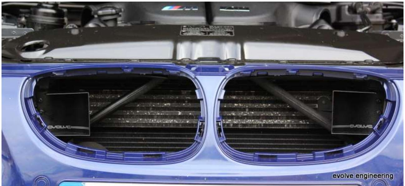
20. Reinstall front grills by aligning tabs and gently pushing. Secure bumper with OEM torx and refit rubber strip.
