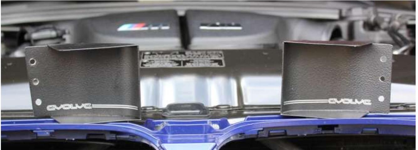
19. Drill 2mm pilot holes with scoops in place and secure with supplied screws:
