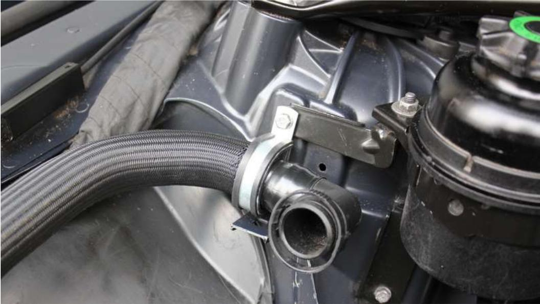
22. Push in supplied breather filter assembly into the secondary air pump tube. This will click into position:
