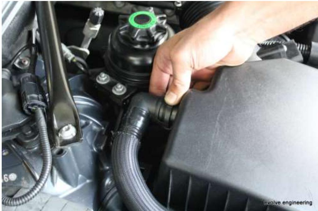
3. Remove upper airbox assemblies by unclipping latches and loosening hose clamps complete with flexible tubing to inlet manifold
