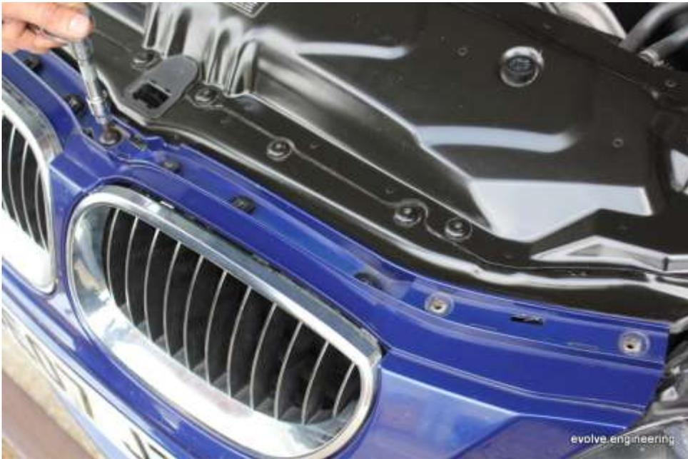
8. Remove both front grills by carefully compressing the clips situated on top and internally
