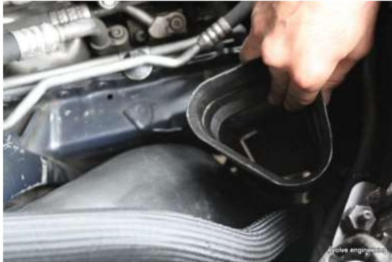
17. Installation of left and right hand heat deflectors:
