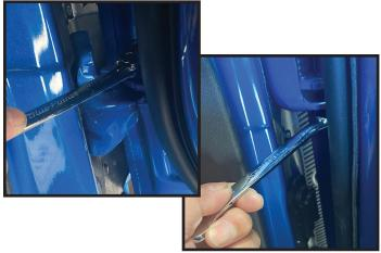
5. Remove the hinge assemblies from the factory door with the 13mm wrench. Transfer the hinges to the composite door and tighten bolts.
