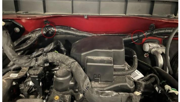
2. Verify the length for connectors thru the openings by the hood hinges, up thru the panels above and to the lights, use edge biter clip zip ties on both driver's side and passenger's side as circled below, cut off the end of zip ties to desired length.
