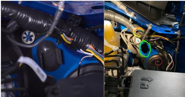
2. Fish wire and switch thru hole and into interior. Be sure to have enough wire going into the interior to reach the desired switch location.
