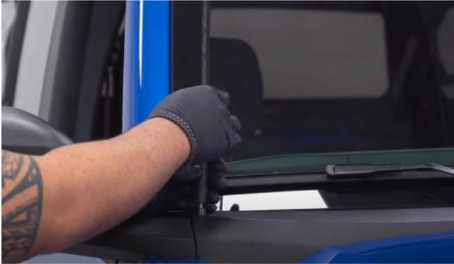
2. Remove the T25 and T30 torx fasteners from the passenger's side of the vehicle. \*Note: The bolt above the antenna is size T30, and the bolt closer to the side mirror is size T25.
