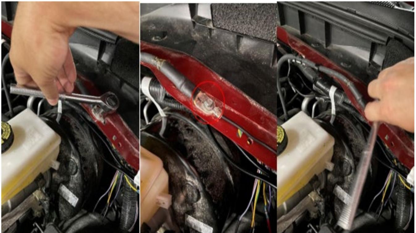
8. Install battery ground (negative) black wire to negative battery terminal.
