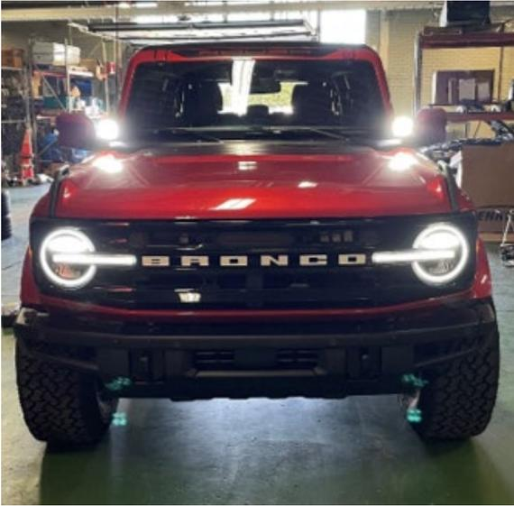
2. Park vehicle in garage with limited or no lighting, move the light bracket to either center position or side position.
