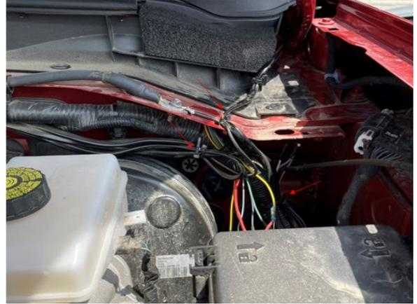
6. Connect the black ground wire and fasten it with 8mm socket to the existing ground on the driver's side rear cowl area.
