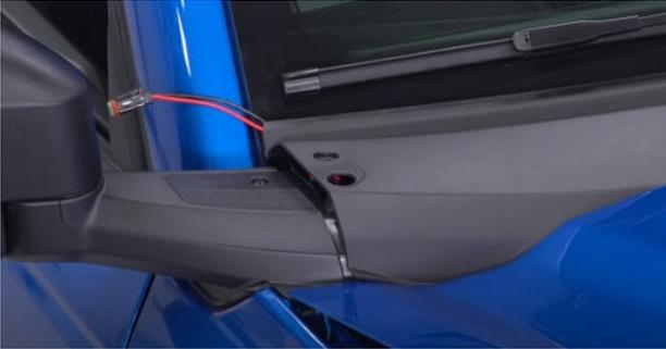
6. While working on the passenger's side, align the Work Light Mounting Bracket in position as shown, tighten down the T25 torx fastener with the supplied washer from the kit.
