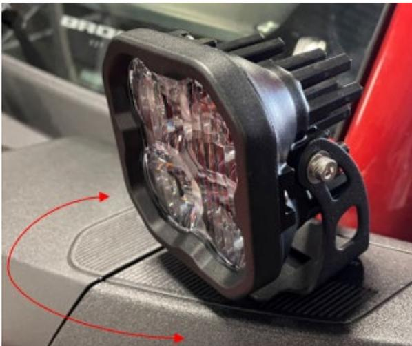
3. Examples below shows the light direction (red arrows) in either center position or side position.
