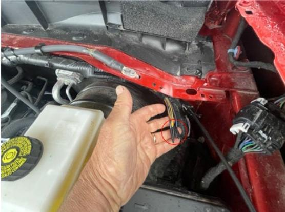
4. Referring to the wiring diagram on the below, locate the yellow wire (1st switch wire).
