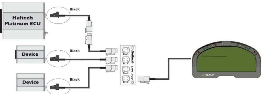
**Figure 10 – Haltech ECU connected to 3 Auxiliary CAN based devices**
