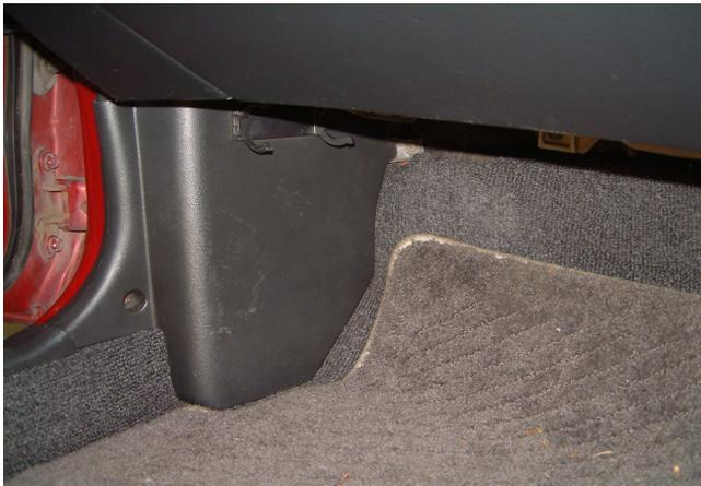
***Figure 7 – Kick panel Re-installed***
