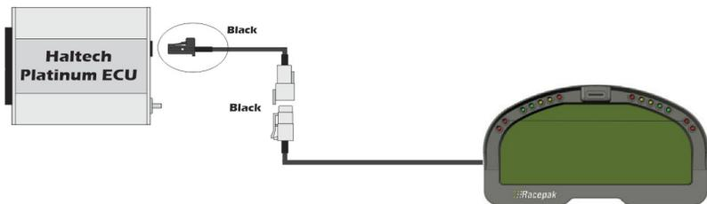
**Figure 9 – Haltech ECU connected to a Racepak Dash**
