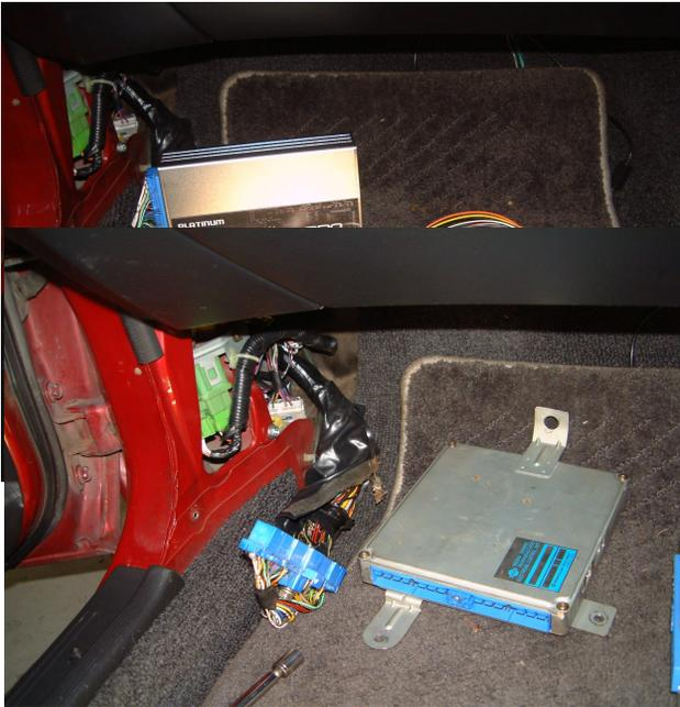
***Figure 3 – Platinum Pro Plug-in ECU Connected,
