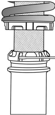
Do not use the adjustment wrench to lock the lower mount, it is only used to adjust the ride height. If the lower locking collar is tightened by the adjustment wrench, it **MAY COME LOOSE**.
