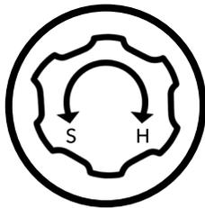
On most vehicles, there is a knob located on the top of the shock which is used to adjust rebound. Rebound is the extending force exerted on the shock after being compressed by a bump or body roll from weight transfer and controls the motion of the car's sprung weight. Use rebound to control the overall handling balance of the car.
