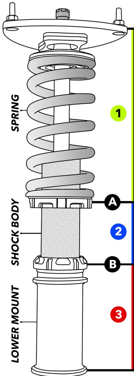
On a true coilover (as shown on the left), always adjust the coilover height from the lower mount (B/3) and NOT the spring perch (A/1). Using the spring perch (A) to adjust the ride height will result in premature wear on the shock and reduce suspension travel. On a divorced rear (as shown on the previous page), the ride height must be set with the rear spring and spring perch assembly.
