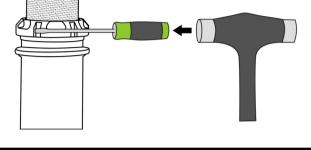
Use a flathead screwdriver and hammer/mallet to lock the locking collar against the lower mount, as shown in the picture.
