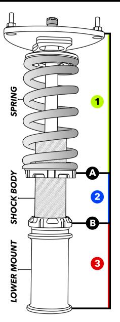
On a true coilover (as shown on the left), always adjust the coilover height from the lower mount (B/3) and NOT the spring perch (A/1). Using the spring perch (A) to adjust the ride height will result in premature wear on the shock and reduce suspension travel. On a divorced rear (as shown on the previous page), the ride height must be set with the rear spring and spring perch assembly.
