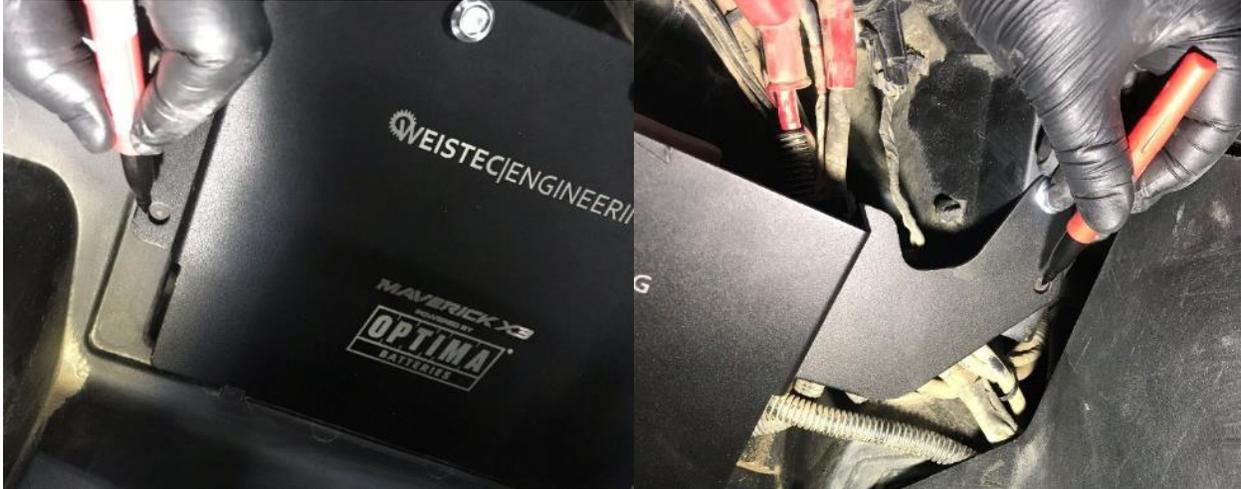
c) Remove the Battery plate and then drill both holes at the marked locations using an 11/32" Drill Bit and Power Drill
