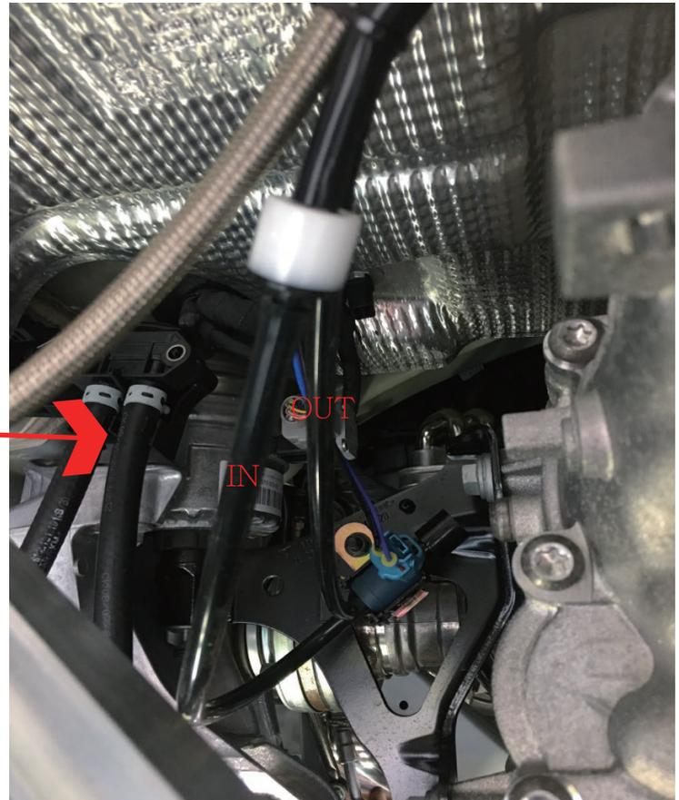
▶ A closer look at where the vacuum source is linked after the 3-way connector is connected
