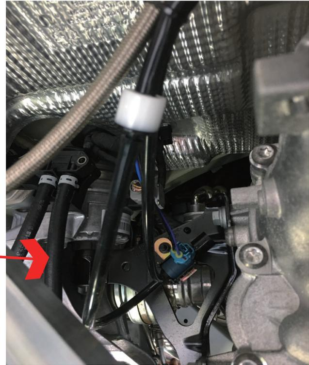
▶ Locate the Solenoid Valve as indicated
