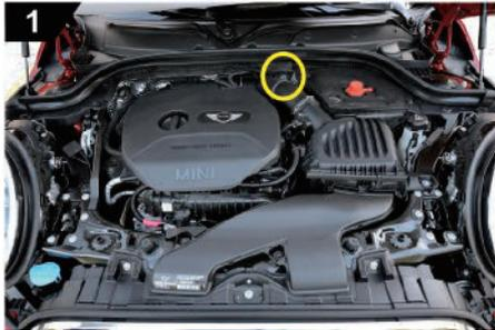
1 Remove the engine cover to reveal connecting location
