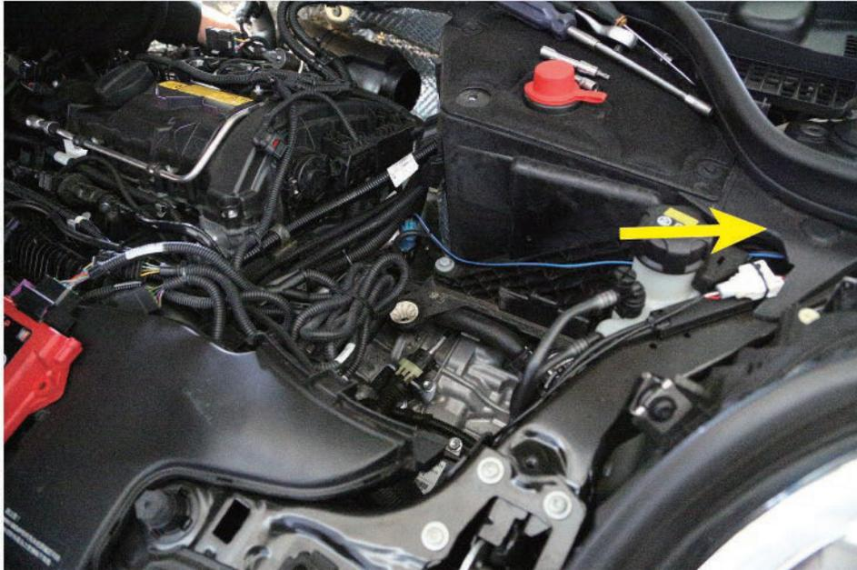
**Direct the Solenoid Wire into the cabin as shown**
