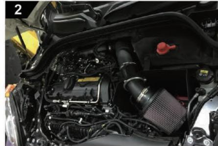
2 Remove the air intake for easier access to wiring
