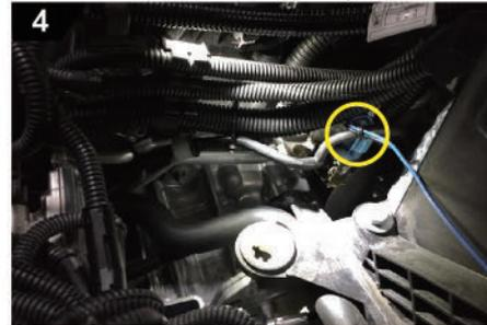
4 Ensure the Solenoid Wire is safely and ssurely connected to the Solenoid Valve
