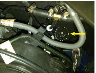
▶ Locate and install the solenoid valve as indicated(beneath).
