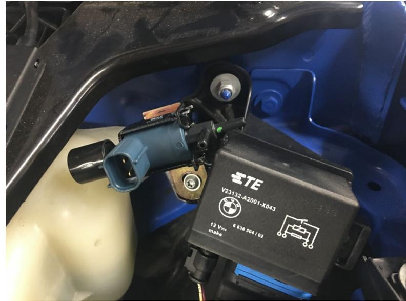
► Install the solenoid valve here
