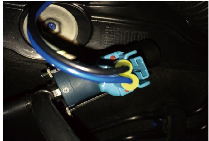
► Securely install the solenoid as shown
