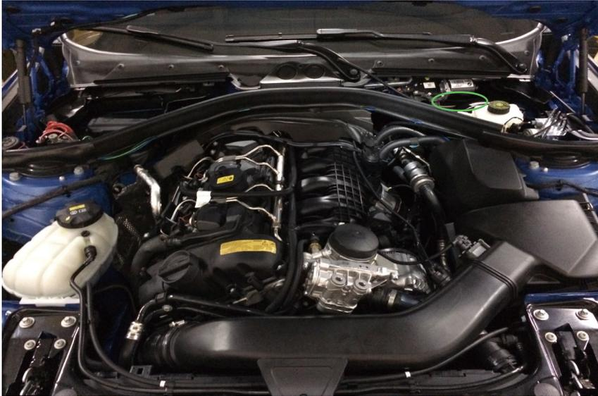
► The vacuum source is located at the top right quadrant of the engine bay
