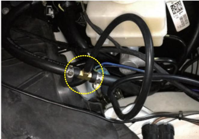
► Install a T-connector to create a vacuum source.
