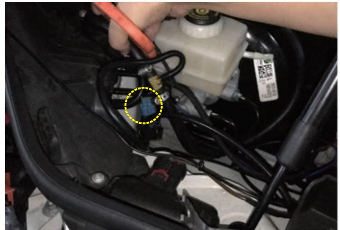
► Locate and install the solenoid valve as indicated.
