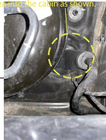
► Install the one-way valve as indicated.
