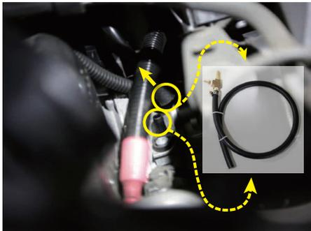
► Connect the vacuum tube as shown.
