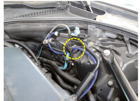
► Install the vacuum tube to the solenoid as shown.
