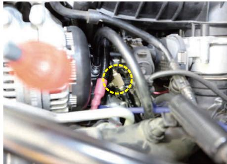
► Install the T-connector and connect the vacuum tube then return it the original position.
