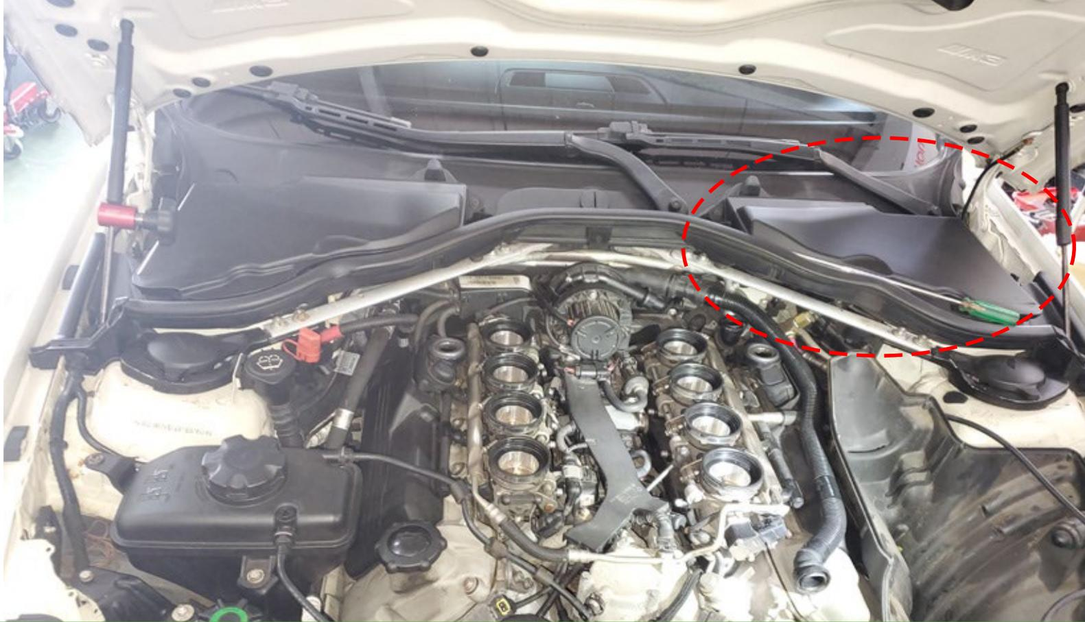
▶ Threading cable from engine bay into cabin For example, threading iron wire from cabin into engine bay and drag cable into cabin
