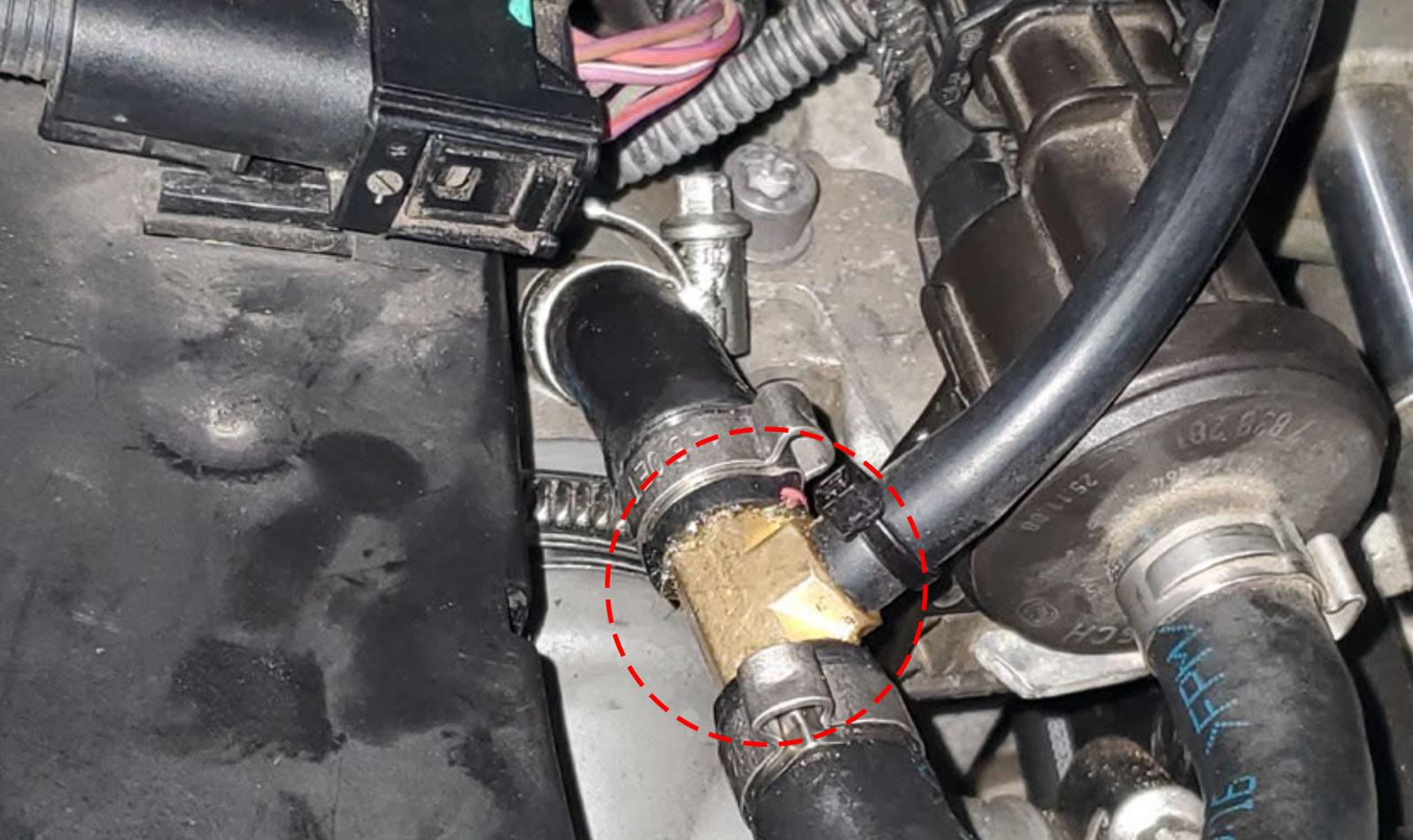
▶ Pull out Original vacuum tube and set up vacuum source
