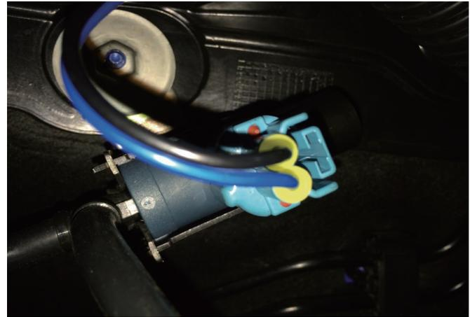
► Securely install the solenoid as shown
