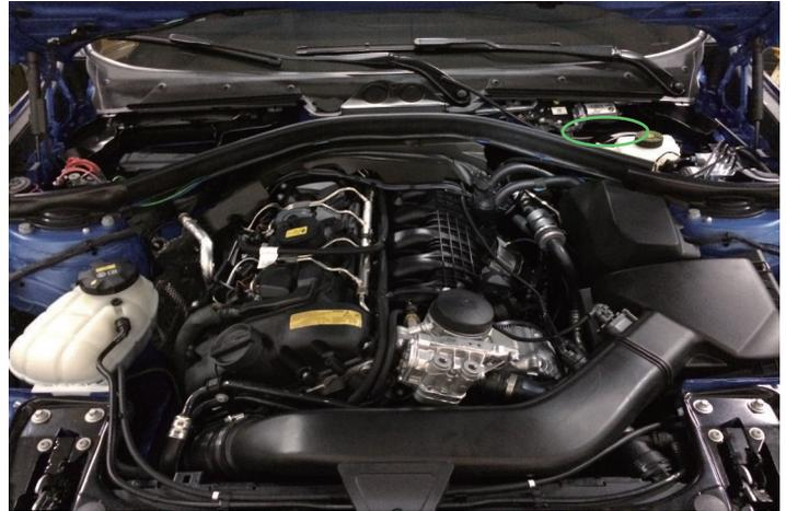
► The vacuum source is located at the top right quadrant of the engine bay
