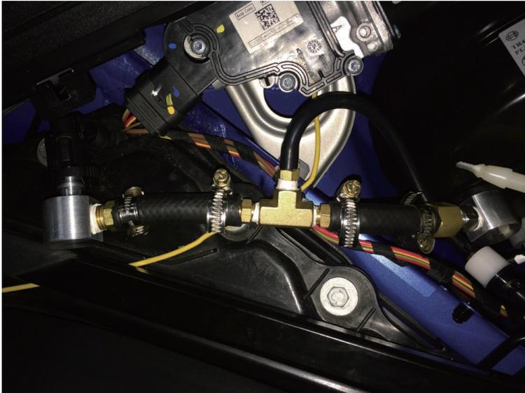
► Remove the stock vacuum tube and connect the T-connector (Apply lubricant when necessary)
