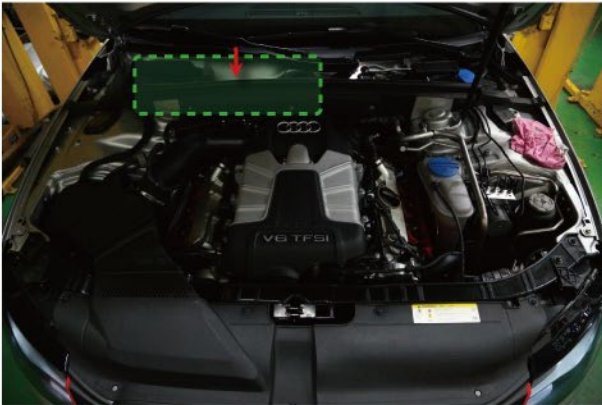
► The solenoid valve is located in the back of the engine bay
