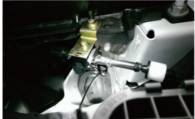
► Close up view of solenoid valve appearance
