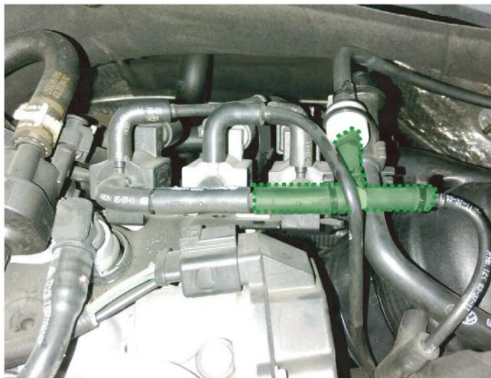
►Detail view of the T-connector location
