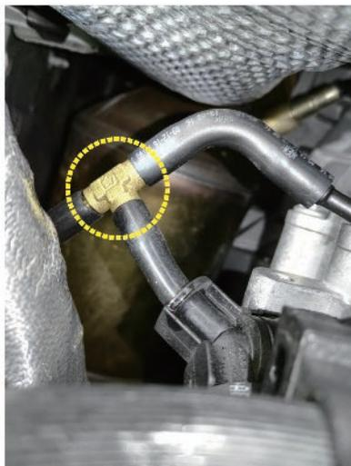
▶ Disconnect the original vacuum tube and install a T-connector to create a vacuum source
