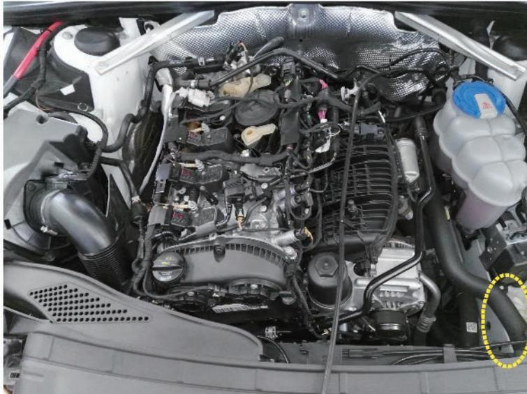
Locate the solenoid valve as indicated
