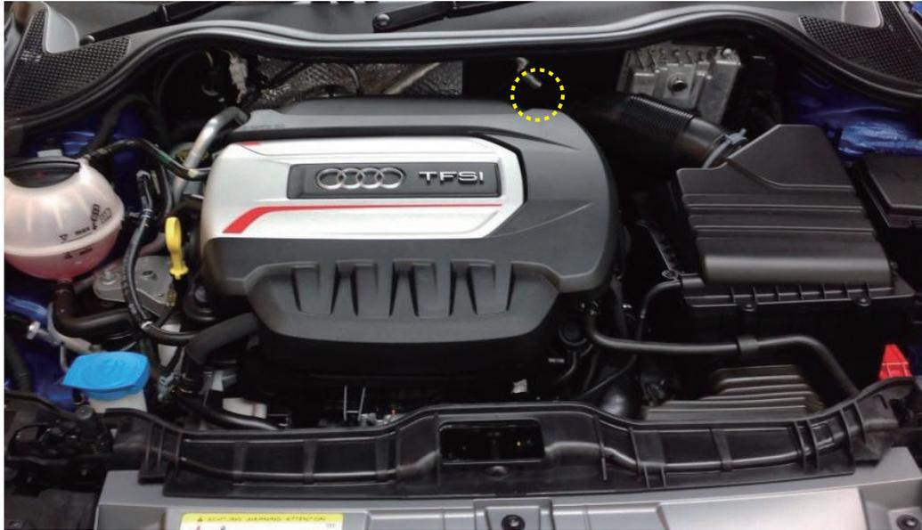
► Locate the vacuum source beneath the intake pipe as shown
