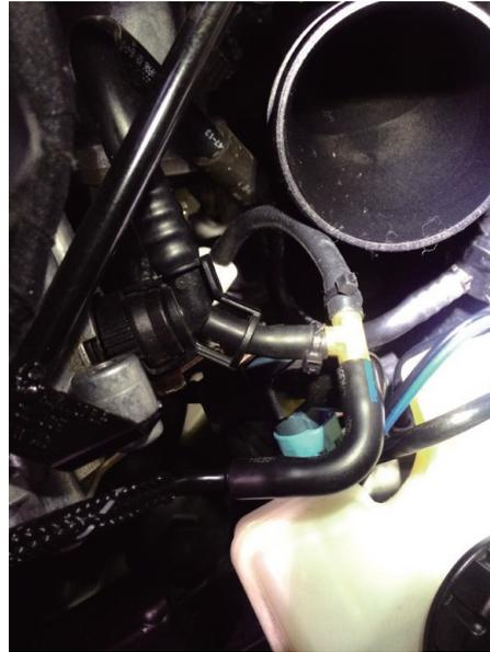
► Remove the stock vacuum tube and install the T-connector and one-way valve
