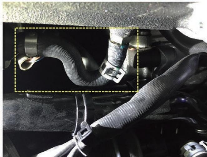
Disconnect the original vacuum tube and install a T-connector to create a vacuum source
