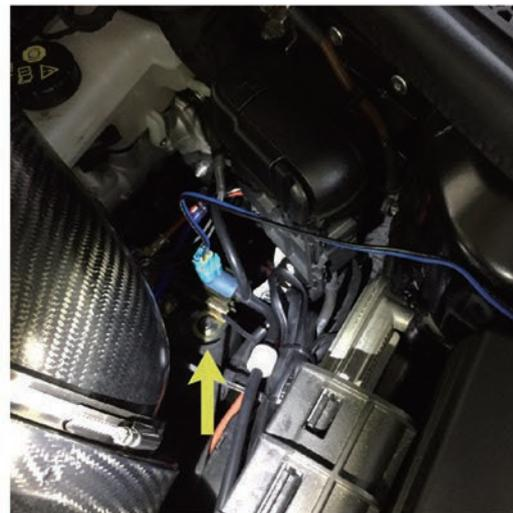
► Install the solenoid valve as indicated
