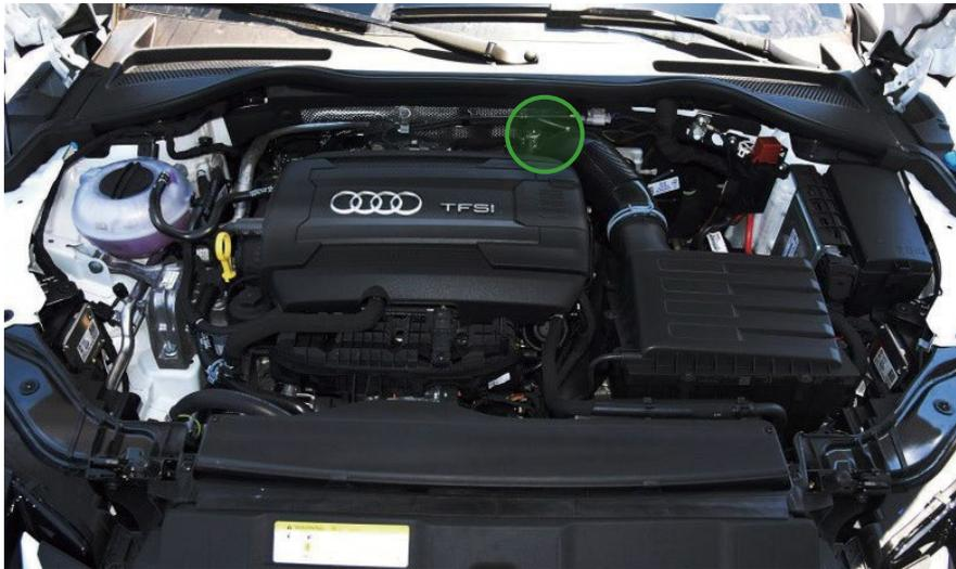
► Locate the vacuum source beneath the intake pipe as shown
