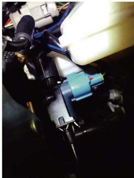
► Secure the solenoid valve beneath the vacuum source and connect the vacuum tube
