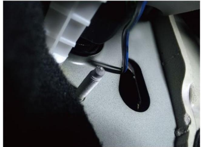
► From above the pedals thread the cable through the rubber opening
