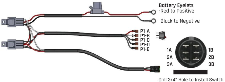
Wiring: Wire your lights according to the instructions included with the light. Take care to avoid any heat sources and sharp or abrasive surfaces.
