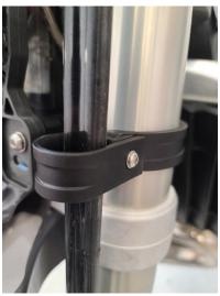
**Note:** Do not fully tighten M4 bolts to allow for adjustment later.
