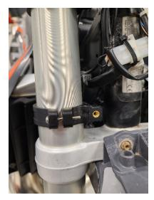
2. Attach P-Clamp (P) to brake line for bottom tube clamp. Use second P-Clamp at upper tube clamp if applicable. Use M4 button socket head and M4 washer (J & K) to secure tube clamps to bike.
