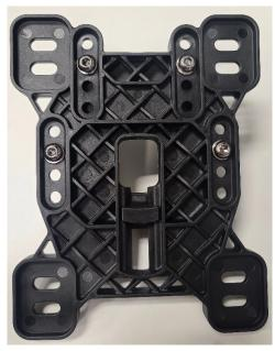
4. Attach bracket plate (S) to tube clamps (N & O) using M6 button socket head bolts and M6 washers (L & M). Adjust each of the clamp heights to line up with one of two slotted holes in each corner of the mount plate.
