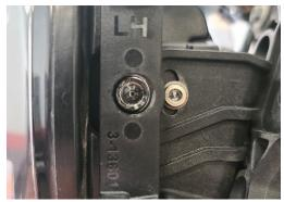
7. Snap number plate onto (4) clips on the light.
