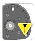
To ensure maximum geometric accuracy, our bushing opening is designed to fit snugly over the factory strut's threaded stud. However, some aftermarket struts or coilover kits may necessitate enlarging the stud hole to accommodate their specific applications.
